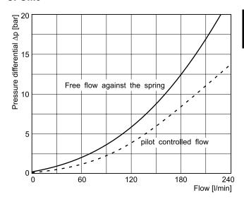
All characteristic curves measured with HLP46 at 50  $^{\circ}\text{C}.$
