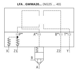
**Control cover "GWMA20"** for set-up of a directional valve: NG25 ... 40 (dimensions in mm)
