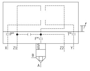
**Control cover "HWMA."** and **"HWMB."** for set-up of a directional valve: NG50 and 63 (dimensions in mm)
