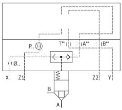
**Control cover "KWMA"** for set-up of a directional valve: NG16 ... 32 (dimensions in mm)
