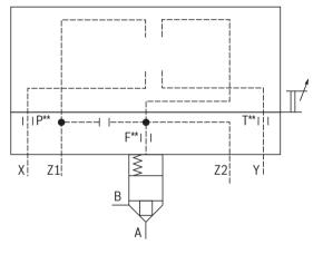
**Control cover "HWMA."** and **"HWMB."** for set-up of a directional valve: NG16 ... 40 (dimensions in mm)
