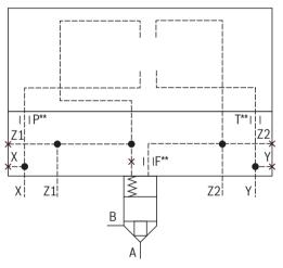
**Control cover "WEMA" and "WEMB"** for set-up of a directional valve: NG63 (dimensions in mm)
