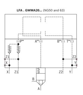
**Control cover "GWMA20"** for set-up of a directional valve: NG50 and 63 (dimensions in mm)
