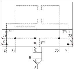
**Control cover "WEMA" and "WEMB"** for set-up of a directional valve: NG80 and 100 (dimensions in mm)
