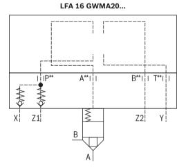
**Control cover "GWMA20"** for set-up of a directional valve: NG16 (dimensions in mm)
