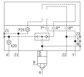
**Control cover "KWMA"** for set-up of a directional valve: NG80 and 100 (dimensions in mm)
