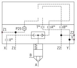
**Control cover "KWMA"** for set-up of a directional valve: NG40 ... 63 (dimensions in mm)
