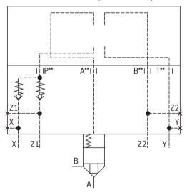
**Control cover "GWMA20"** for set-up of a directional valve: NG80 and 100 (dimensions in mm)
