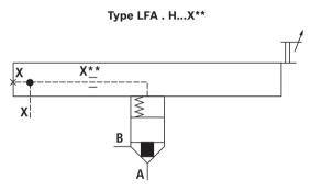
**Control cover "H."** with stroke limitation and remote control port: NG50 and 63 (dimensions in mm)
