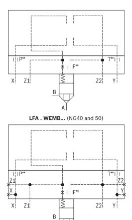
**Control cover "WEMA" and "WEMB"** for set-up of a directional valve: NG16 ... 50 (dimensions in mm)
