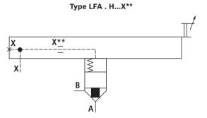
**Control cover "H."** with stroke limitation and remote control port: NG16 ... 40 (dimensions in mm)
