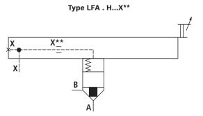
**Control cover "H."** with stroke limitation and remote control port: NG80 and 100 (dimensions in mm)
