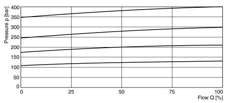
All characteristic curves measured with HLP46 at 50  $^\circ\text{C}.$
